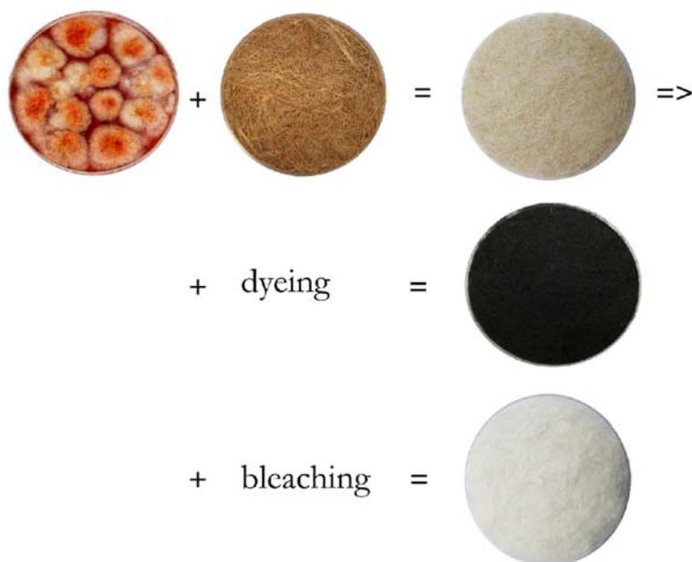
Figure 1. The principle of Fusart®-method
