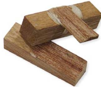
Fig 7. Positive test result showing timber fracture of modified sample.
