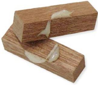
Fig 6. Negative test result showing adhesion failure (adhesive delaminating from wood surface) of non-modified sample.
