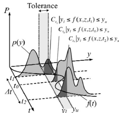
Fig. 2 Concept of the robustness index for adjustable control factor
