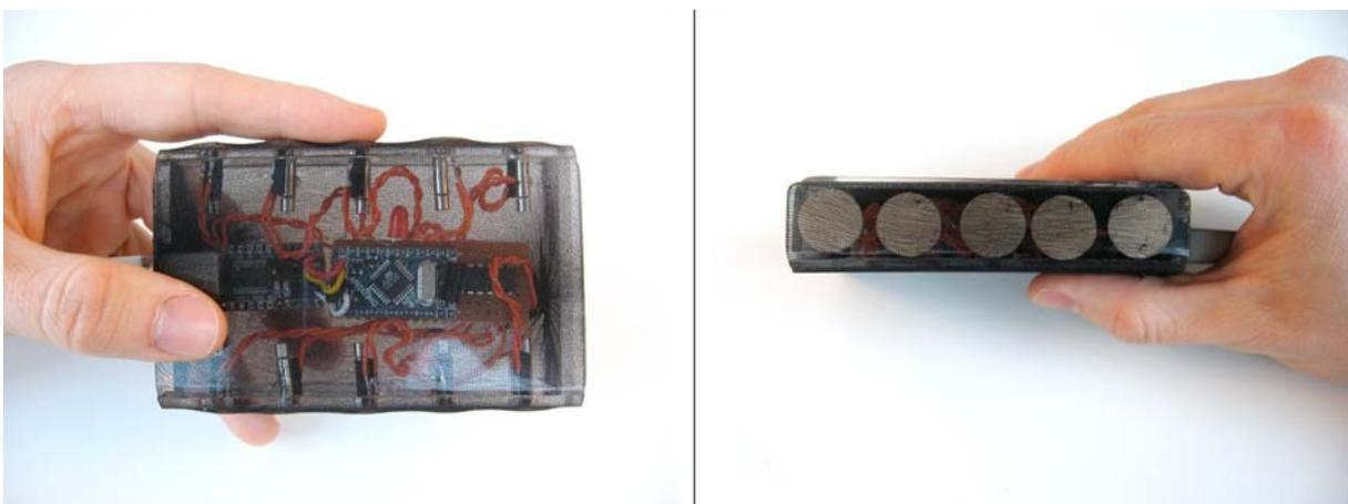
Figure.2 Grip with 10 vibrotactile disks, controlled over USB
