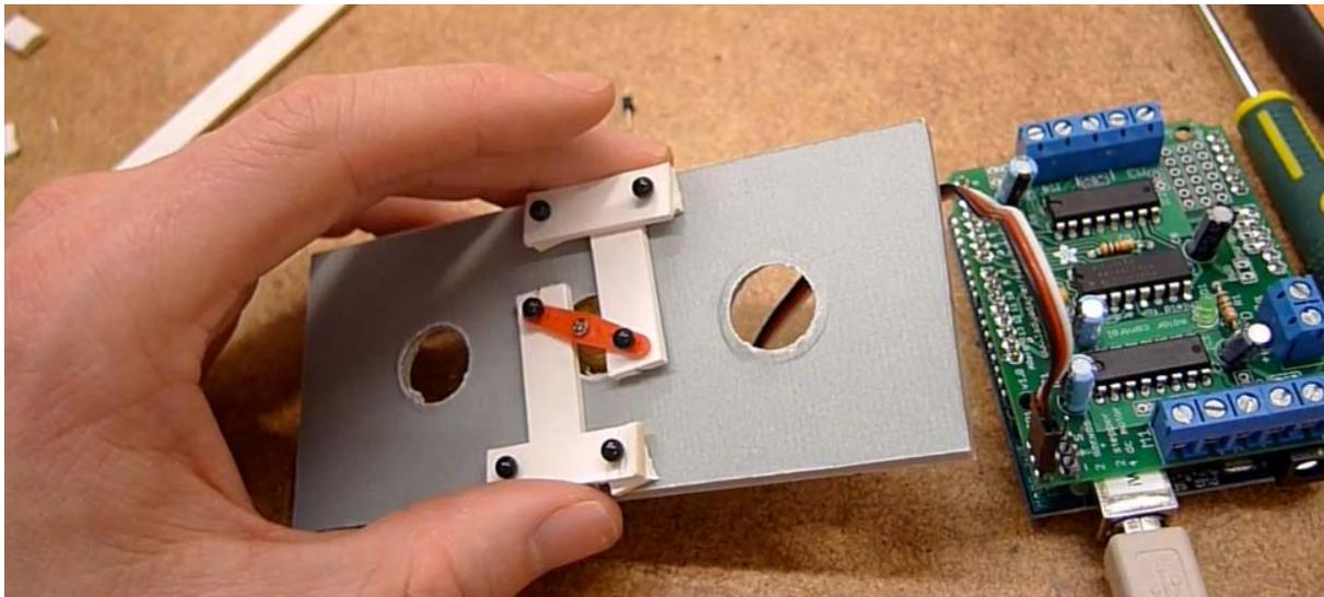
Figure.5 Quickly building a cardboard haptic device
