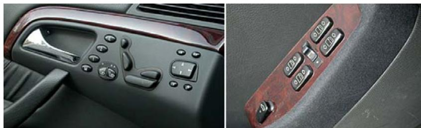
Figure. 2 Seat adjustment control and window switch from a Mercedes-Benz<sup>6</sup>
