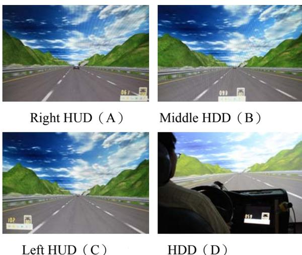
Figure 1: Speed-limit messages on the display of IVIS
