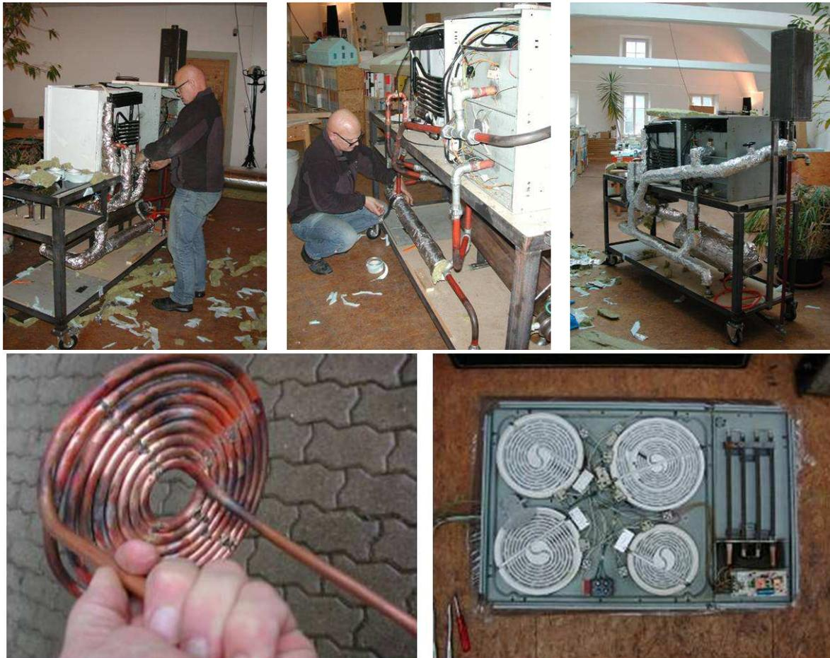
Figure 5. Prototyping of a thermal oil based refrigerator and cooking stove [16] (Pictures: Atelier Schmidt)
