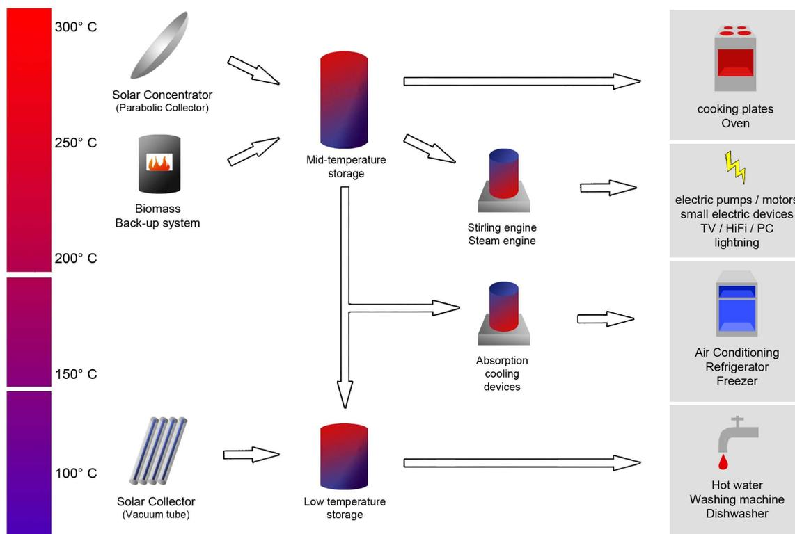
Figure 2. Solar thermal energy supply system of Wireless House [16]
