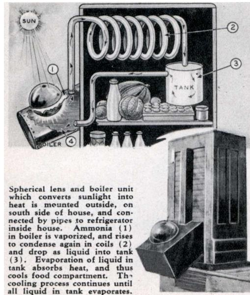
Figure 3. Early solar-thermal based refrigerator designs [10]
