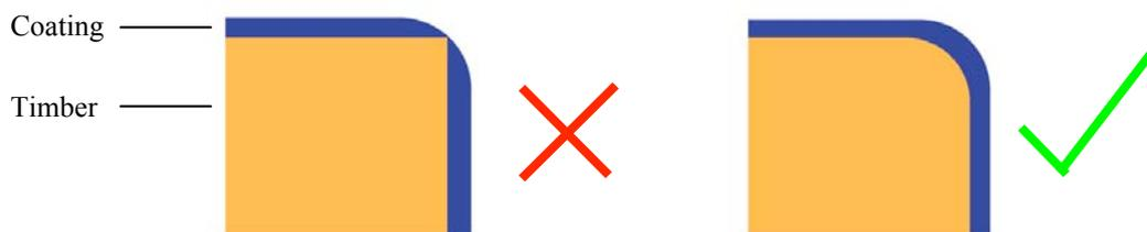
Fig 10. A visual example highlighting the importance of incorporating a radius on a right-angled edge.
