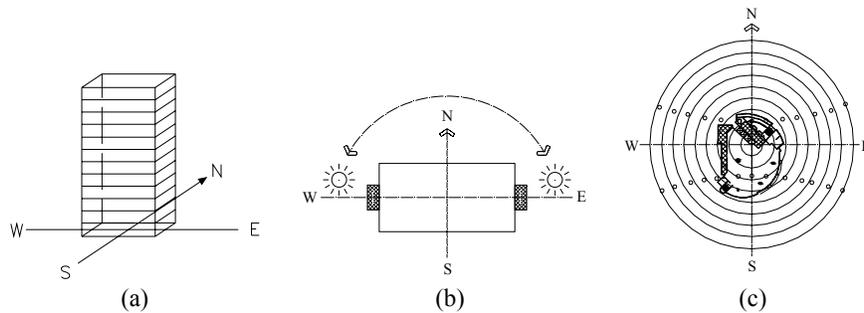
Figure. 3 (a) Fitting orientation of the urban high-rise housing in Vietnam; (b) Service cores on the hot sides of built form; (c) Sun path and HCMC tower designed by Ken Yeang [17]
