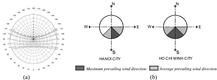
Figure. 2 (a) Sun path in HCMC [3]; (b) Direction of the prevailing wind in Vietnam
