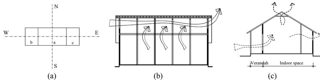
Figure. 1 (a) Main part of folk house typical; (b) Cross ventilation through two air-holes in lengthwise section; (c) Ventilation in the cross section
