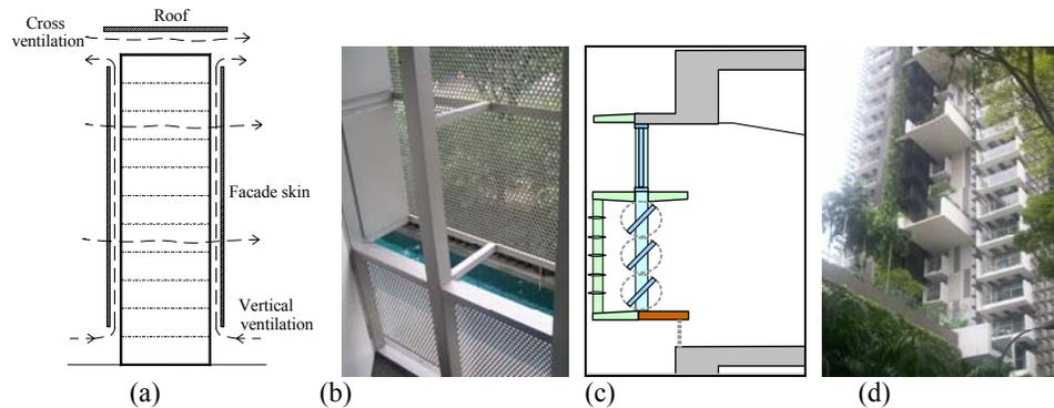
Figure. 4 (a) Vertical and cross ventilation model for the building envelope; (b) Horizontal ventilation and vertical sun-screening on the South facade of the Moulmein Rise, Singapore; (c) Controllable window [5]; (d) Protruding balconies in the Newton Suites, Singapore.
