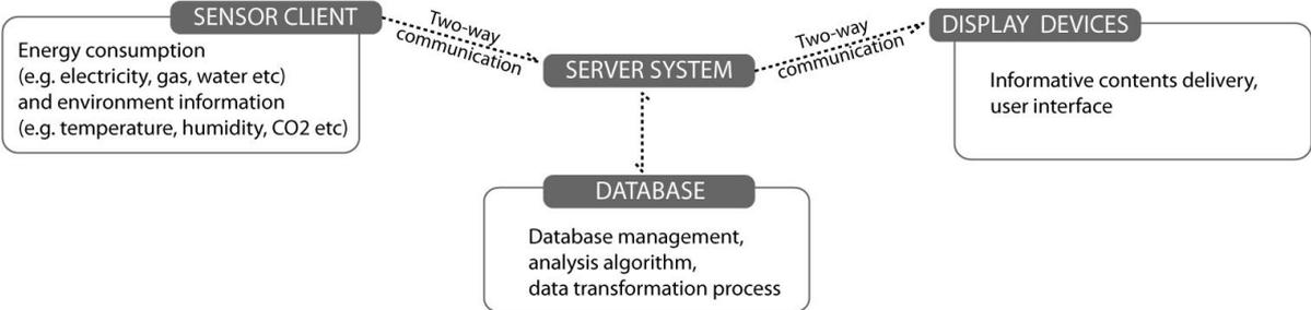
Figure.1 Schematic diagram of on-line energy feedback system.
