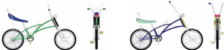
Fig 2. The front view and side view of Idea 1 and Idea 2
